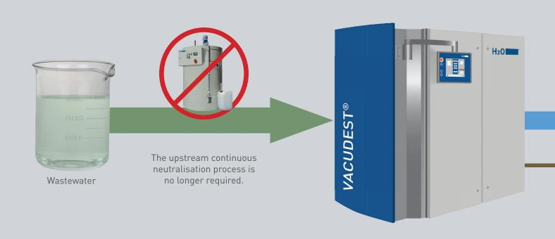
The Destcontrol can be used anywhere which requires constant distillate qualities for circulation processes. It is particularly suitable for alkaline or slightly acidic water, and replaces conventional continuous neutralisation, e.g. during wastewater processing in paint pre-treatment or aluminium die-casting.
