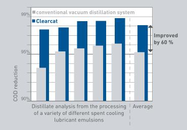
The Clearcat condensation system stands for crystal clear distillate, including a COD reduction improved by 60 percent compared to conventional evaporators.
