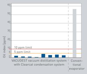
The future proof Clearcat condensation system allows better reduction of the oil index than conventional evaporators combined with post treatment steps.
