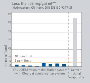
The future proof Clearcat condensation system allows better reduction of the oil index than conventional evaporators combined with post treatment steps. This allows the oil content to be reduced to less than 38 mg/gal.
