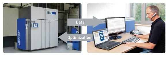
Efficient process optimization: The Vacutouch control system allows direct VACUDEST process data transfer to our technical customer support.
