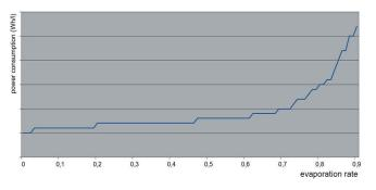
Power consumption of vacuum distillation systems depending on evaporation rate
