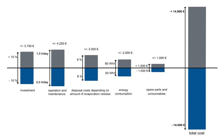
Fig. 1: Variation of operation cost of vacuum distillation systems.
